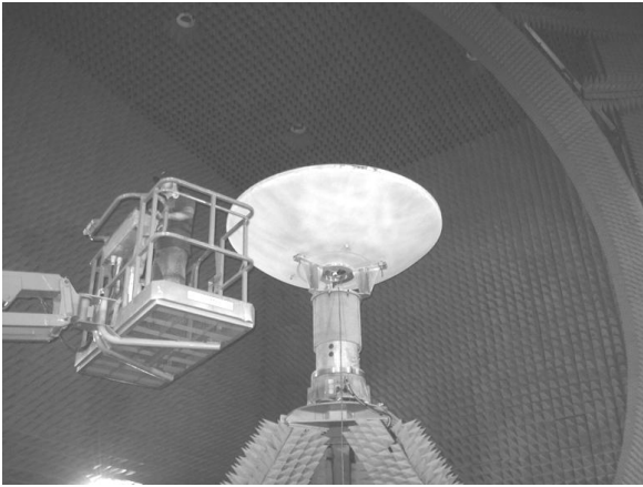
Figure 8 The AUT as mounted in the SNFR prior to pattern testing
